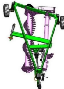
Shipping kit installed ready for truck
